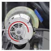
Correct shaft rotation is clockwise.
