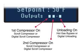
Typical display for chillers with a discus compressor and a capacity unloader.
