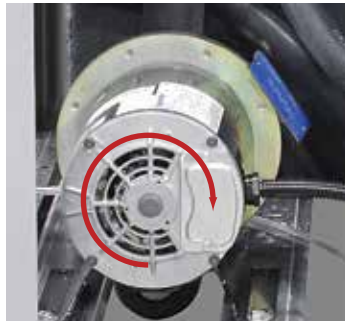
Correct shaft rotation is clockwise.
