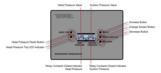
E. When either the head pressure or suction pressure is measured out of the set point range the corresponding arrows will disappear. If the head pressure is out of range the red LED will come on and the reset button will have to be manually pushed after the condition has been corrected.
