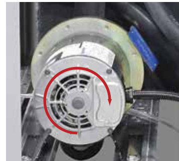
Correct shaft rotation is clockwise.
