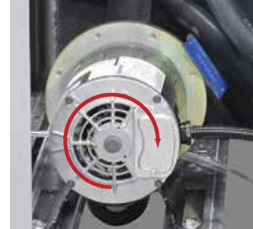
Correct shaft rotation is clockwise.
