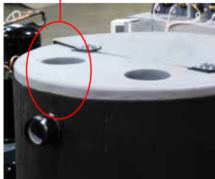
Typical reservoir lid and From Process opening.
