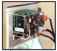
B. **TRANSFORMER.** The transformer supplies 110 volts to the controlling instrument (figure 6.2B).
