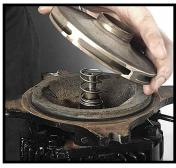
Aligning impeller and spring
