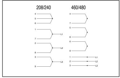
Wiring schematics for 240 and 480 volt pump motors
