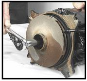
Removing impeller locking screw with ratchet Figure 5.1H
