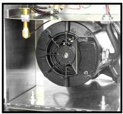
Remove shaft cover to view Figure 3.2B the motor shaft
