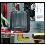
Panel mounted pressure switch Figure 3.2A
