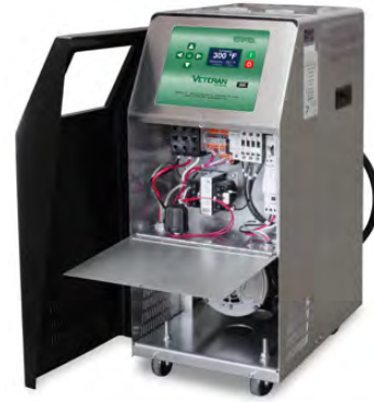
Thermoformed panel removed and electrical cabinet open.
