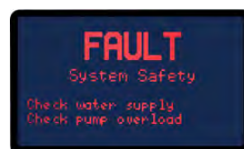
System Fault Screen. Indicates a water supply or a pump overload fault.
