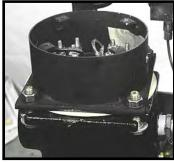
Heater mounting bolts Figure 5.2C
