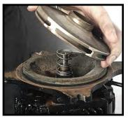
Aligning impeller and spring
