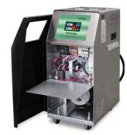
Thermoformed panel Figure 5.5A removed and electrical cabinet open.
