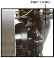
Electric Pump Figure 6.1A Motor Adapter
