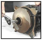
Removing impeller locking screw with ratchet
