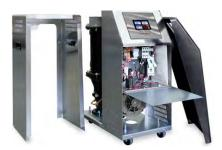
Thermoformed panel removed and electrical cabinet open.
