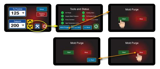
**5.** Press the Stop button to disengage the purge cycle. Use the Back back to return to the Tools & Status screen.
