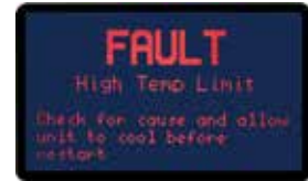
High Temp Limit Fault Screen.
