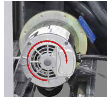
Correct shaft rotation is clockwise.
